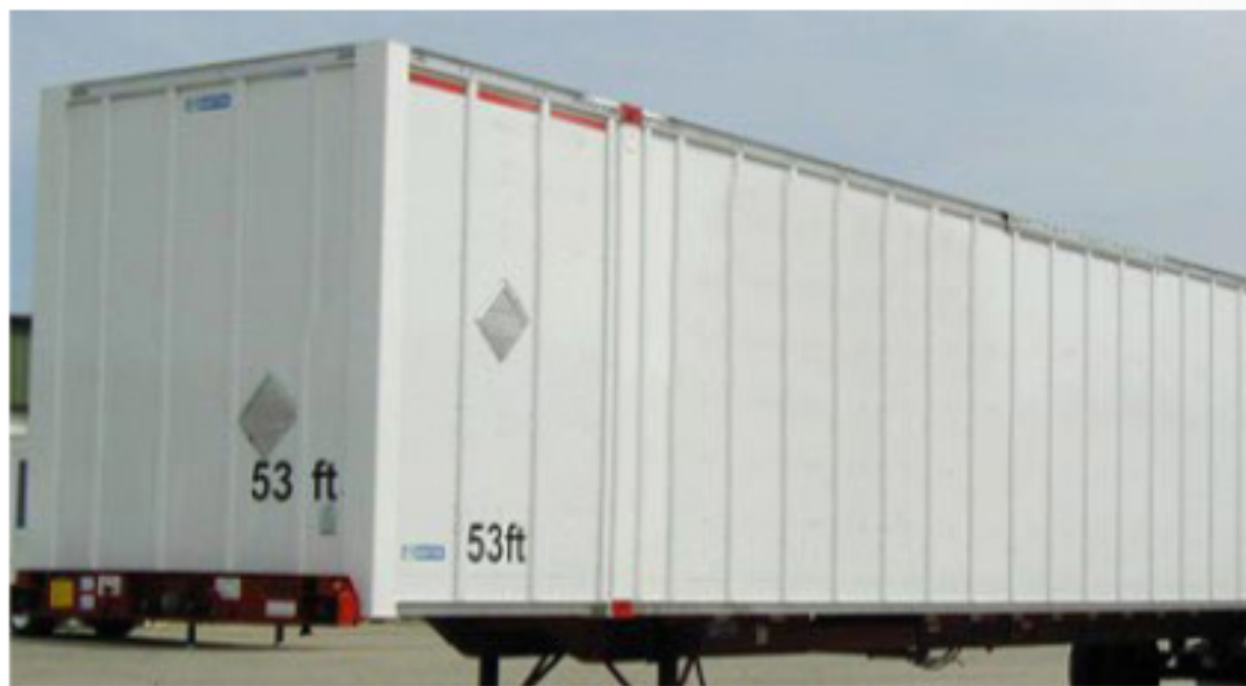
STEEL CLAD COMPOSITE PANEL
