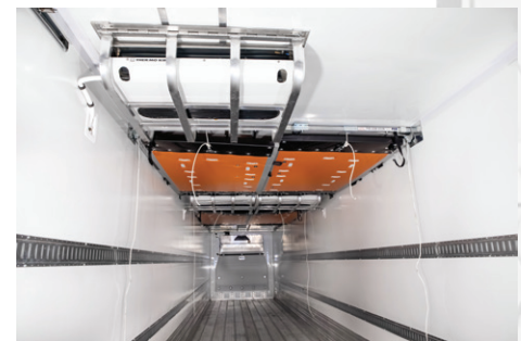
Multiple bulkheads and evaporators create specific temperature zones
